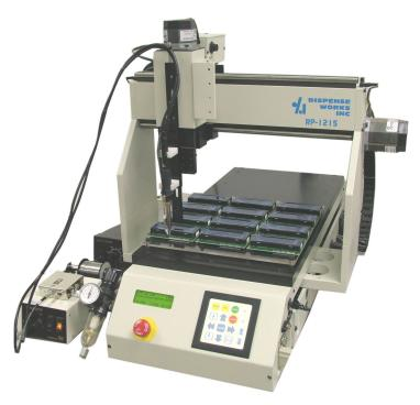
The versatile RP-1215 Robot is the perfect platform for tooling with its large, flat 12" x 24" base plate. Product remains stationary, only the head moves from overhead. Pre-Loaded lead screws and ball slides in each axis provide the accuracy and rigidity for successful solder joints and high thru put speeds.
